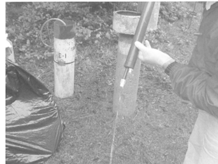
AIR IS THE ENEMY: Air can adversely affect a sample. The pictured bladder pump has oxidized because of air intrusion.
