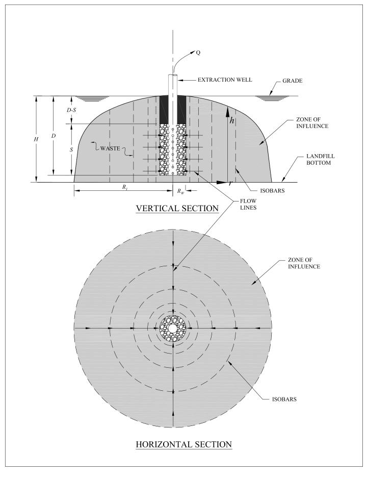
FIGURE 1. VERTICAL LFG EXTRACTION WELL MODEL
