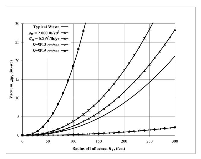
FIGURE 2.  $\Delta \psi$  VERSUS  $R_I$  FOR VARIOUS WASTE TYPES
