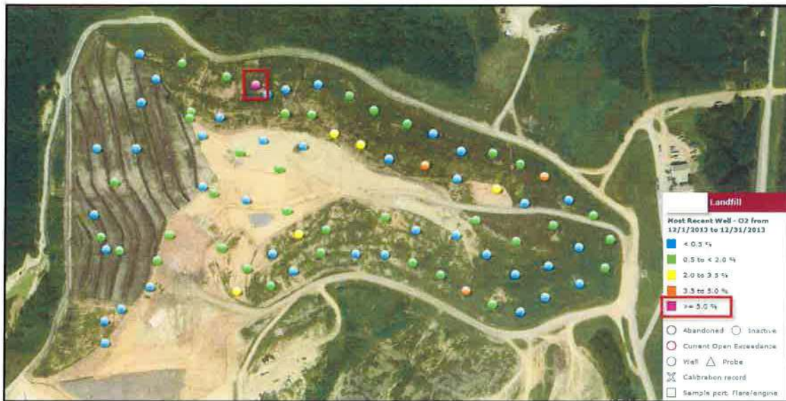
Figure 1. LFG Extraction Well Oxygen Concentration Range Map, Site A
