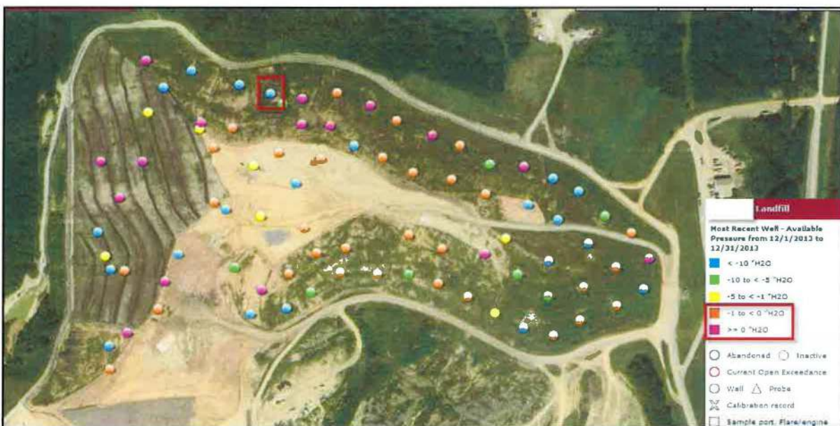
Figure 3. Wellhead Available Pressure Map, Site A
