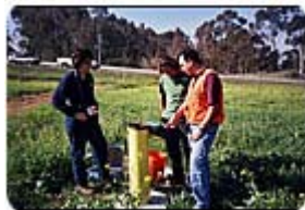
The perimeter and interior probes were monitored for gases using a Landtec GEM 500 Gas Extraction Monitor.
