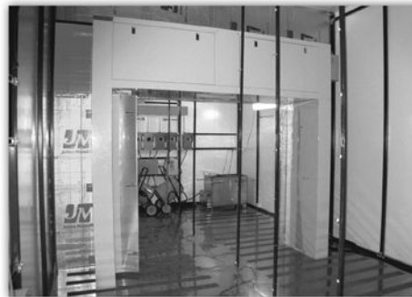
The HCR calorimetric environmental test chamber at CTS Labs in Urbana, IL
