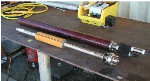
Figure 6 – CEE Liquid Extraction Pump
