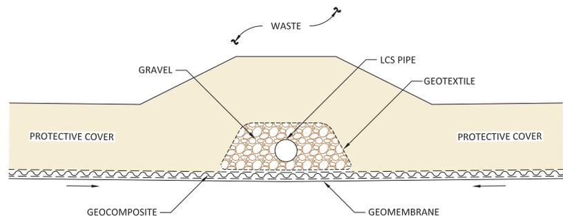
FIGURE 1. LEACHATE COLLECTION SYSTEM WITH A POTENTIAL FLOW BOTTLENECK
