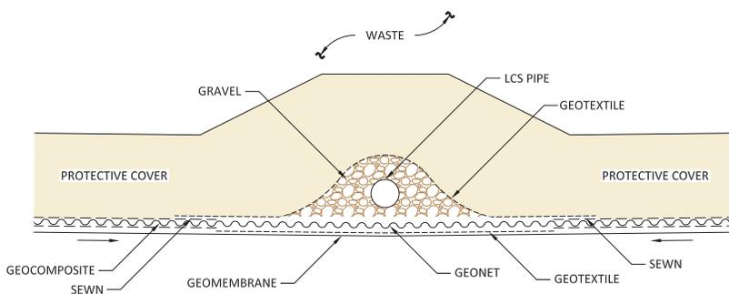
FIGURE 2. LEACHATE COLLECTION SYSTEM WITH NO FLOW BOTTLENECK
