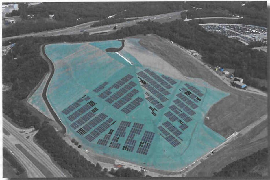
**Figure 2:** Exposed geomembrane landfill cap with laminated solar photovoltaic panels provides power to serve 224 homes. Photo courtesy of Carlisle Energy Services, Carlisle, PA, [www.carlisleenergy.com](http://www.carlisleenergy.com).
