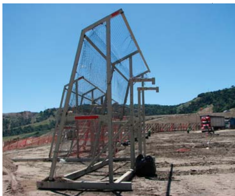
FENCED IN: Portable litter fencing is in use throughout the country to prevent blown landfill litter from being carried off site.
