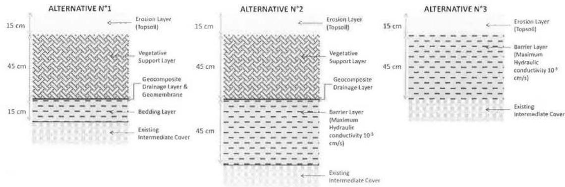
Figure 1 Alternative capping systems assumed for simulations with HELP and LWB models.
