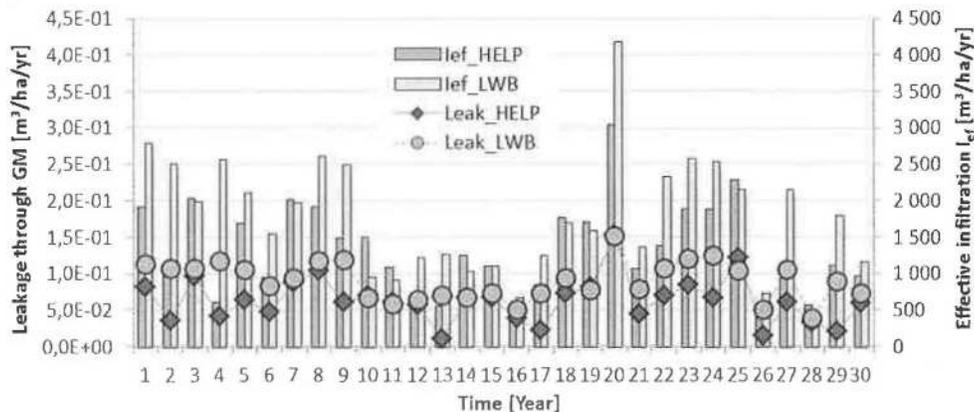
**Figure 2** Annual trend of effective infiltration (bars) and leakage through GM (symbols) provided by the HELP and LWB models for the capping system N°1.
