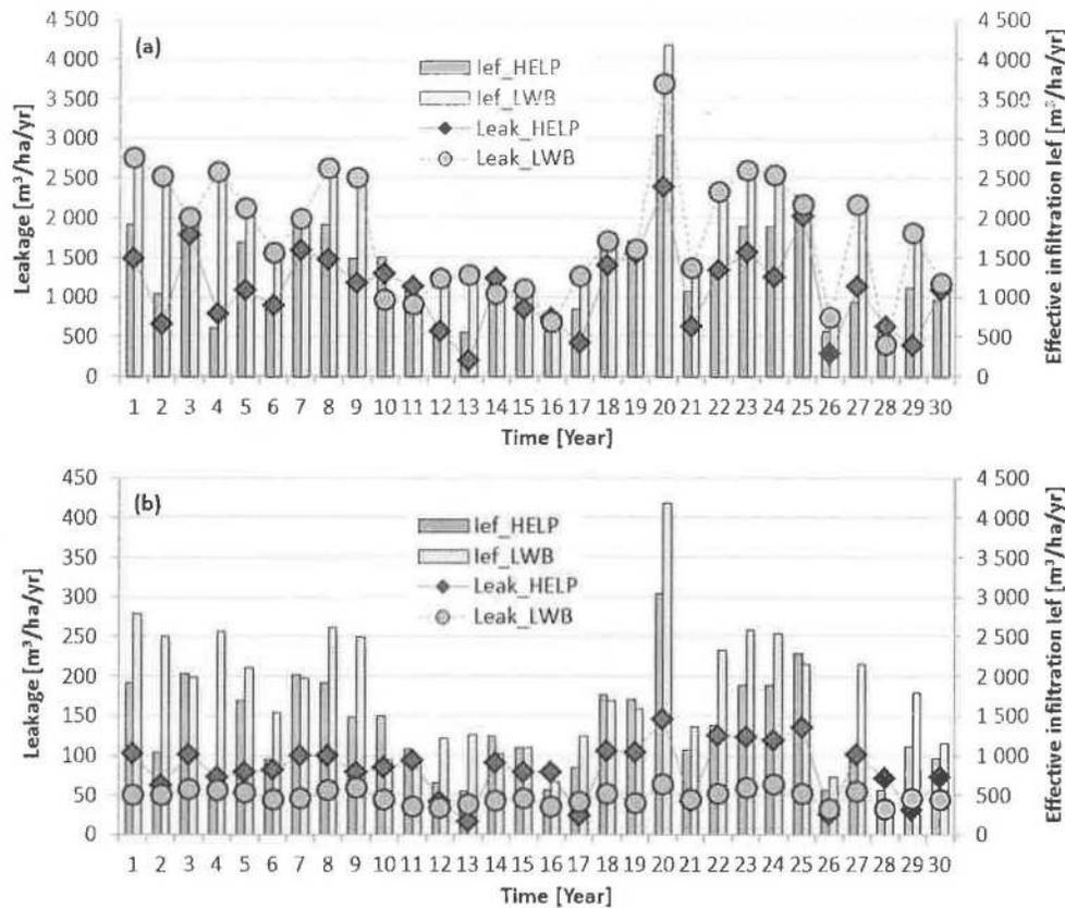
**Figure 3** Annual trend of effective infiltration (bars) and leakage through GM (symbols) provided by HELP and LWB models for the capping system N°2, assuming the hydraulic conductivity of clay of  $10^{-5}$  cm/s (a) and  $10^{-7}$  cm/s (b), respectively.
