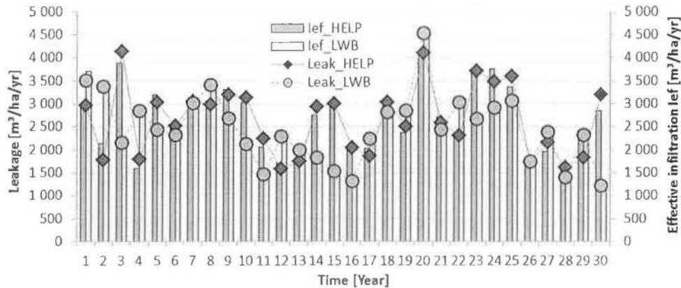
Figure 4 Annual trend of effective infiltration (bars) and leakage through GM (symbols) provided by the HELP and LWB models for the capping system N°3, assuming the hydraulic conductivity of clay of  $10^{-5}$  cm/s.
