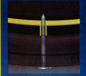
Goodyear DuraSeal Technology is the world's first built-in tire sealant that helps keep fleets running puncture after puncture, even after multiple retreadings.
