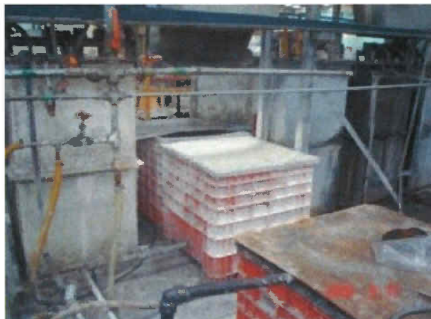
Figure 3: Corroded floor beneath the plating operation . Clarifier sumps were used to contain plating fluids and acids.
