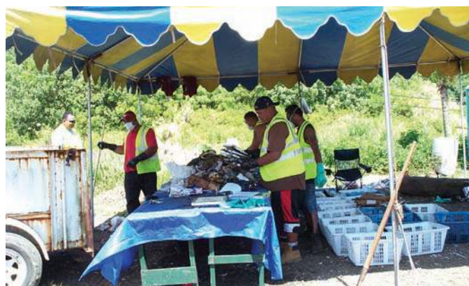
Waste loads were separated by a team of sorters into more than 50 different categories and then a Btu value of the entire waste stream was calculated.
