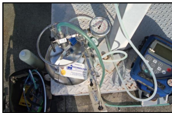
SAMPLE TRAIN WITH SUMMA CANISTER DURING ONE OF THE THREE SAMPLING EVENTS.
