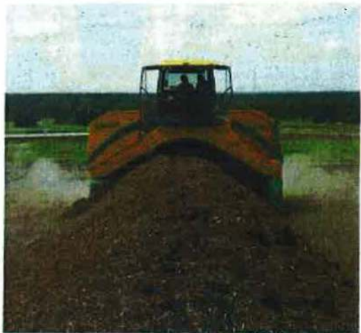
The pilot tested the Modified Static Aerobic Pile™ method, where active windrows sit undisturbed for about 30 days, then are turned twice (Backhus straddle turner above) to assure moisture distribution and material consistency. After 45 to 60 days of curing, the county used a Doppstadt trommel (right) to screen finished compost.
