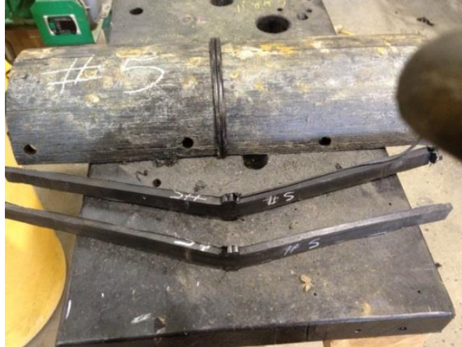
Figure 6. Bend back test on perforated HDPE Pipe
