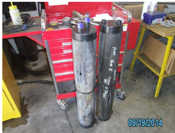
Figure 7. Hydro test on non-perforated HDPE Pipe
