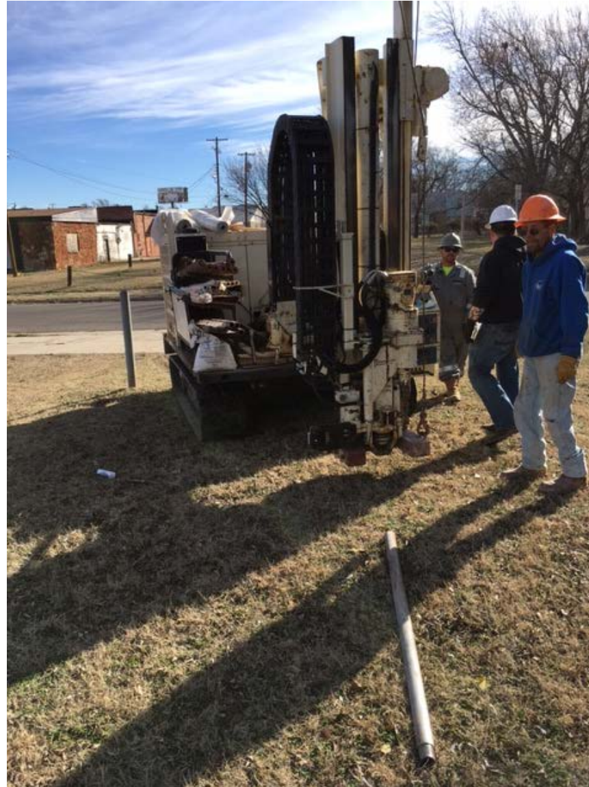
Single-rod direct-push at SS-01
