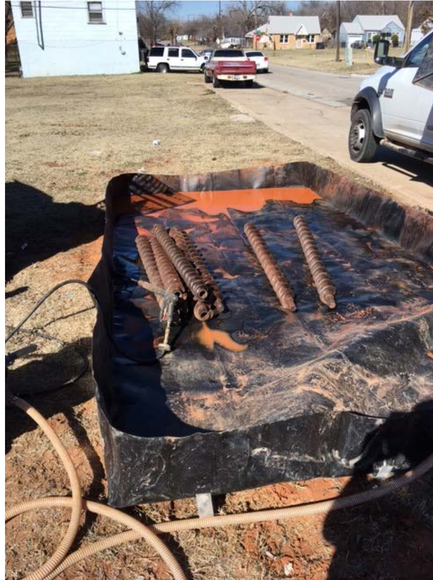
Decontamination of solid-stem flight between soil borings
