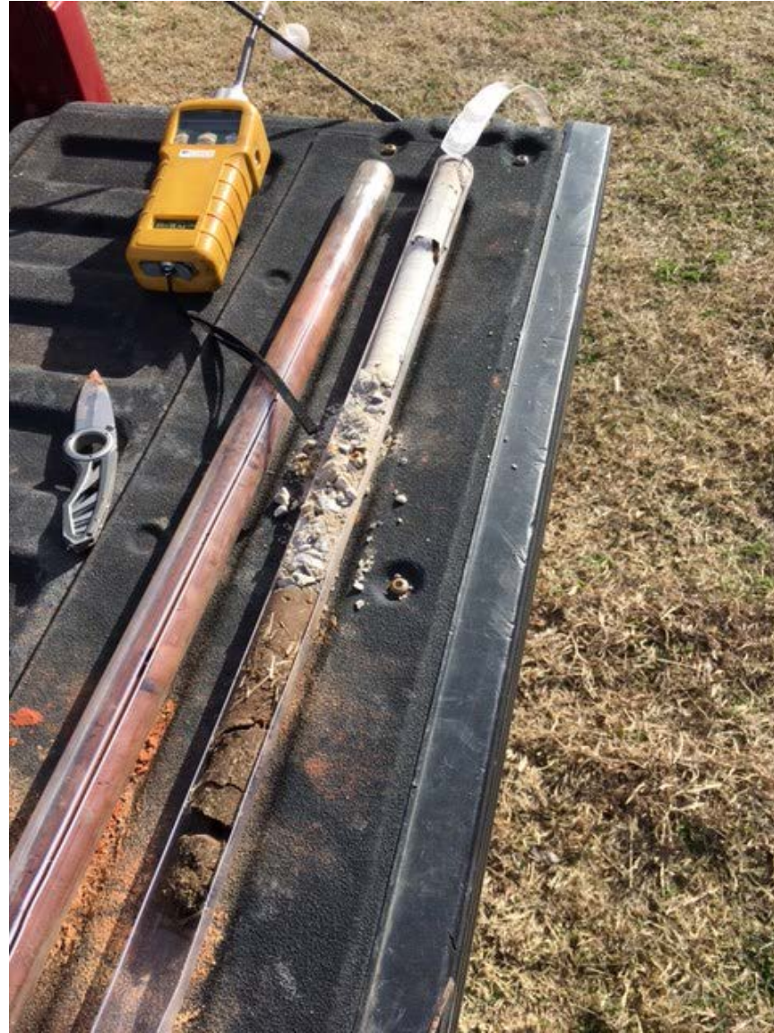
Soil cores in acetate liners
