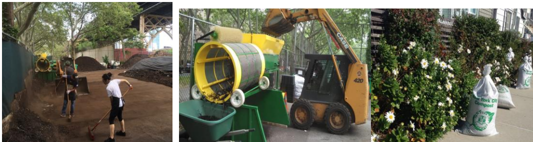
Figure 4. Screening process and final bagged product
