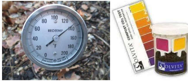
Figure 5. Temperature probe, Solvita Maturity Test
