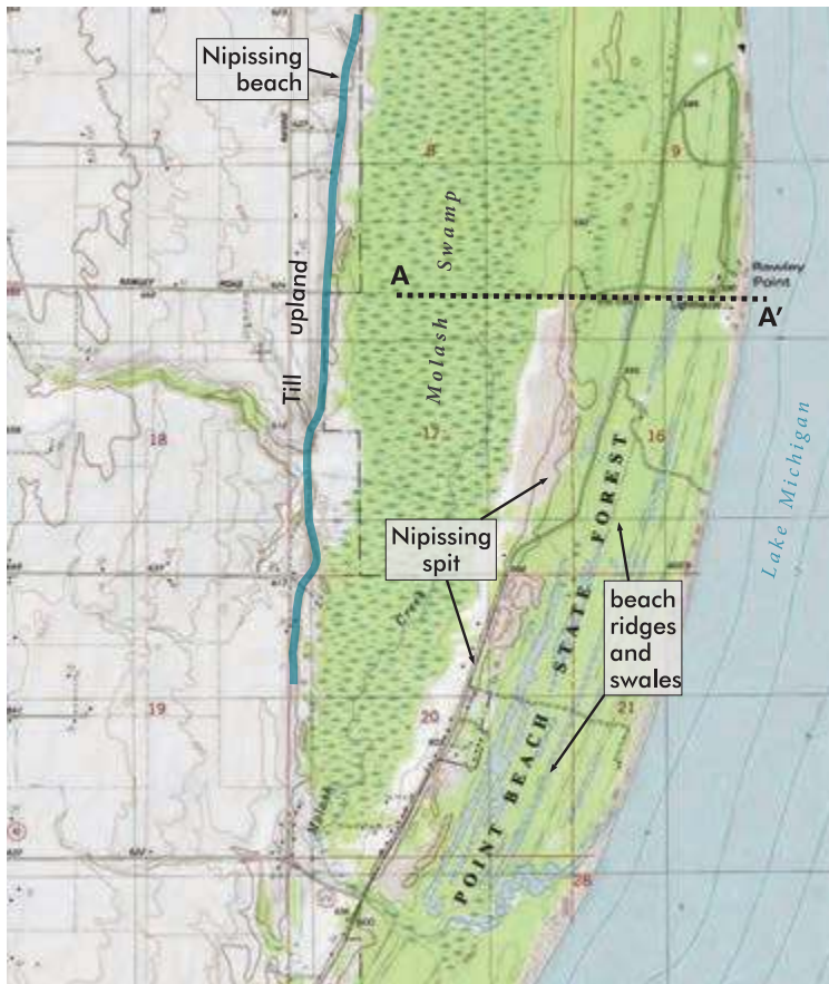
Figure 25. Topographic map of Point Beach State Park (part of Two Rivers 7.5-minute quadrangle). The eastern edge of till upland (blue line) marks the shoreline during the Nipissing highstand of the lake. At that time the spit was built by migrating sand and the Molash Swamp was a lagoon that slowly filled with organic deposits. Dotted line (A-A') shows location of cross section in figure 26.
