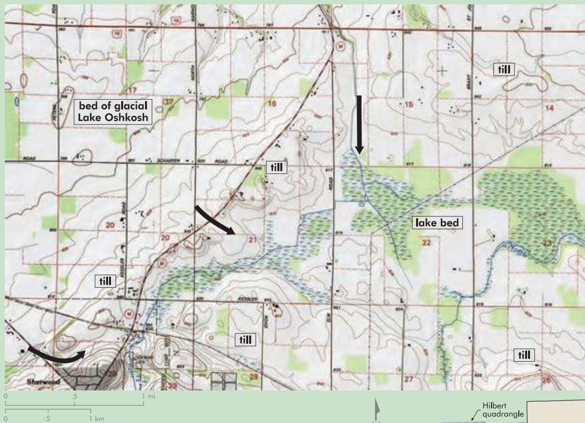
Figure 21. Topographic map (parts of Hilbert and Sherwood 7.5-minute quadrangles) showing the three shallow channels (arrows) through which water from glacial Lake Oshkosh flowed into the Manitowoc River outlet.
