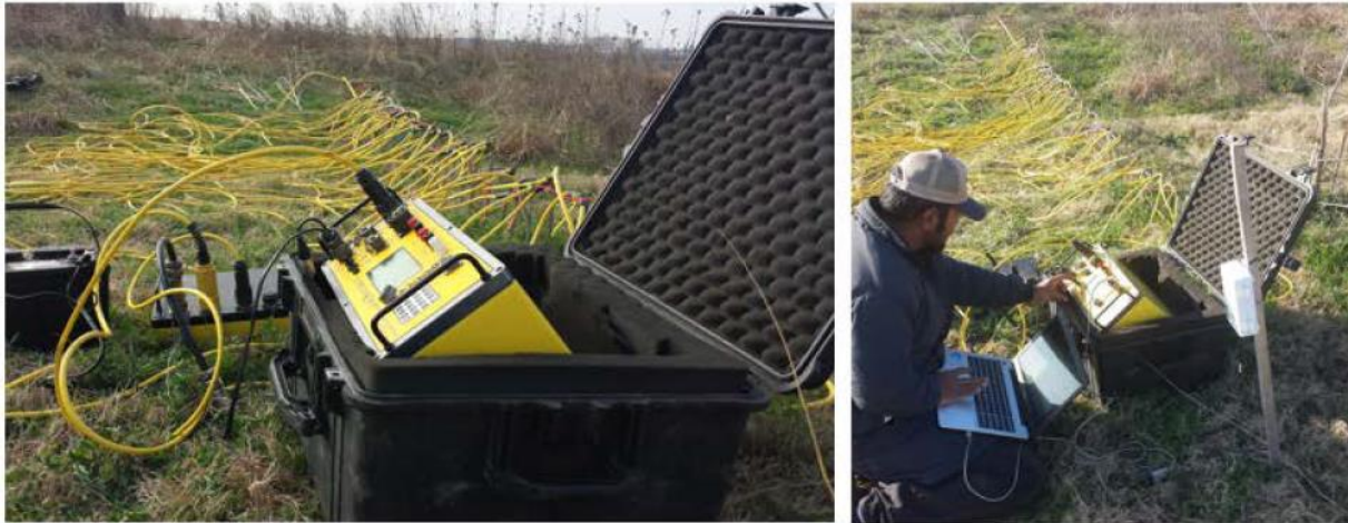
Figure 2. Field setup with resistivity meter and testing
