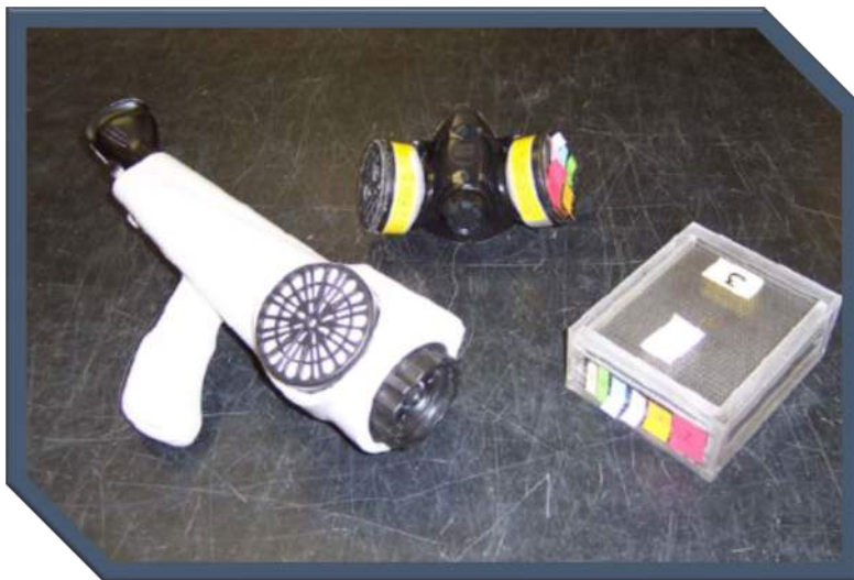
Figure 3: Examples of Field Olfactometers (Nasal Ranger, Facial Mask, Box Scentometer)
