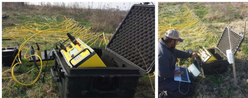
Figure 2. Field setup with a resistivity meter and testing
