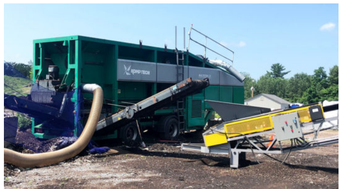
A star screen equipped with a windsifter located on the improved surface area on top of the sand pit.
