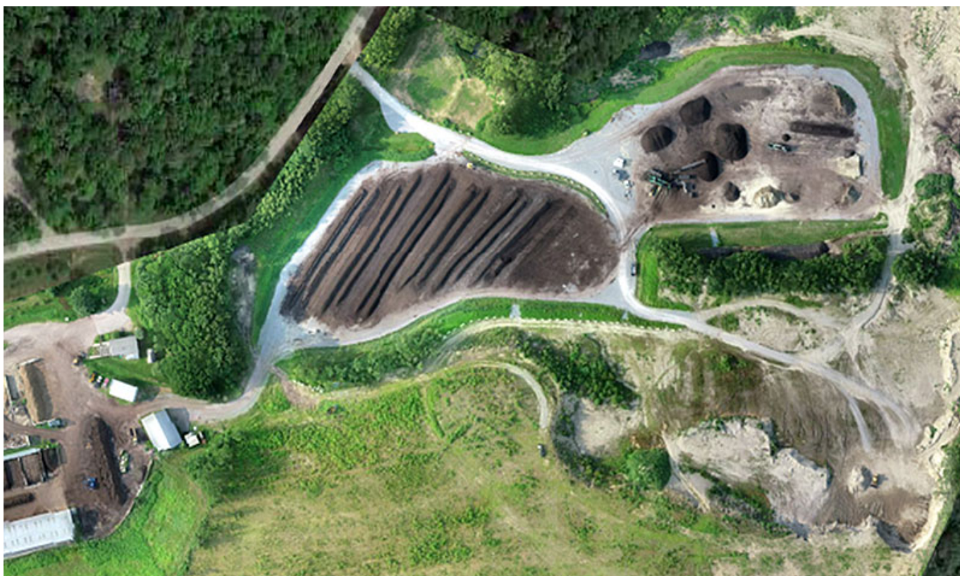
The new windrow composting pad (center) and screening/retail yard (upper right) are on about 7 acres of improved surface. The covered bunkers and a portion of the aerated static pile pad are visible in the lower left corner. Photos courtesy of Green Mountain Compost
