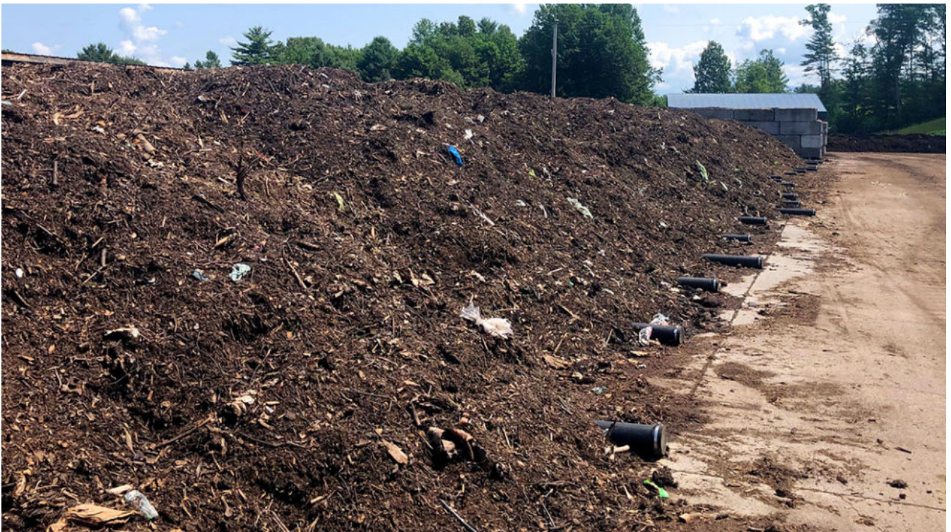
The second phase of active composting is done on an open pad with moveable, above ground aeration pipes. Residence time in Phase 2 is three weeks.
