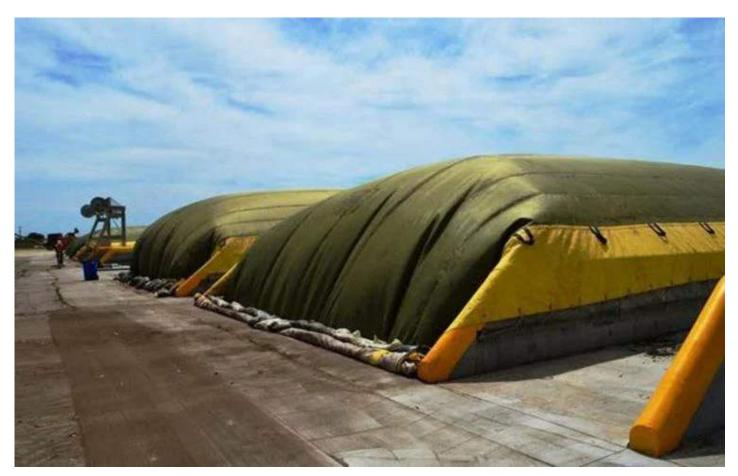
A micro-pore structure made by Gore allows water vapor, air and carbon dioxide to escape from composting operations. Meanwhile, the fabric captures other gaseous materials including volatile organic compounds and ammonia, which are then recycled back into the composting process and broken down by microorganisms.
