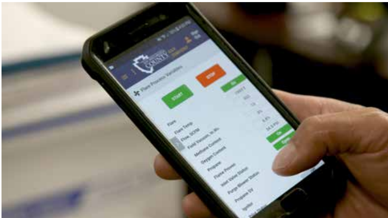
The mobile application lets San Bernardino County control SCADA from anywhere. Courtesy: Inductive Automation
