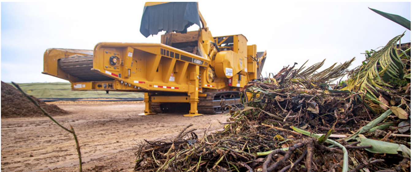
Incoming organic materials are size-reduced in a horizontal grinder to a particle size of about 3 to 4 inches.
