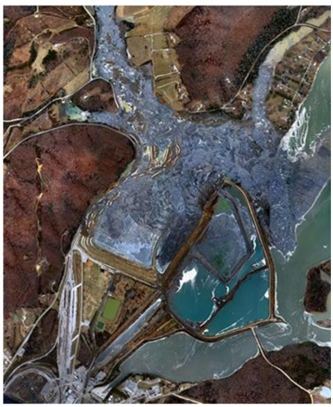
1. Sometime around midnight on Dec. 22, 2008, a dike at the coal ash dewatering pond for the TVA's 1,400-MW Kingston power plant failed. It led to what has been called the largest industrial spill in U.S. history. Source: TVA
