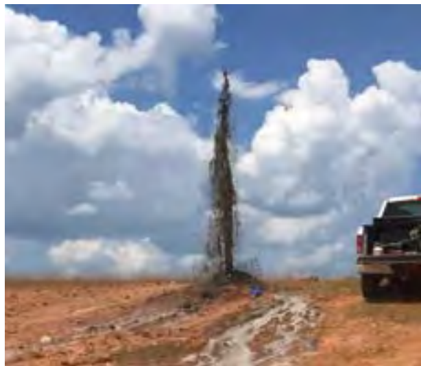
Figure 1 - Excess pressure/liquids inside wells can result in geyser conditions.
